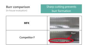
Cutting conditions: Vc = 180 m/min, fz = 0.3 mm/t, ap × ae = 3 × 78 mm, dry, workpiece: GGG60
