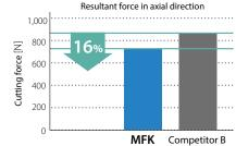
Competitor A Cutting conditions: Vc = 180 m/min, fz = 0.3 mm/t, ap × ae = 3.0 × 62 mm, Dry, Workpiece : GGG60, ø125
