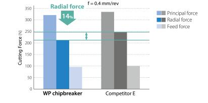
Cutting conditions: Vc = 200 m/min, ap = 0.3 mm, wet Toolholder: A20R-SCLCR09-22AE Insert: CCMT09T304 type Workpiece: 15CrMo4
