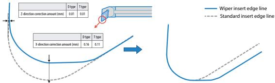
Programming correction is necessary for plunging with D and T type inserts (Not necessary for up-facing)
