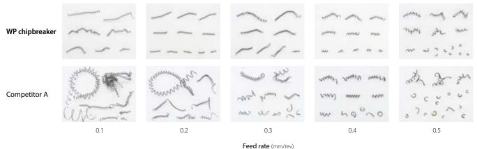
Cutting conditions: Vc = 200 m/min, ap = 0.3 mm, wet Toolholder: A20R-SCLCR09-22AE Insert: CCMT09T304 type Workpiece: 15CrMo4
