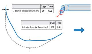
For D type and T type, program corrections are required for ramping and profiling
