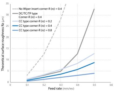
The theoretical surface roughness of a wiper insert is lower than inserts without a wiper
