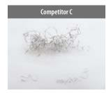
Cutting conditions : Vc = 400 m/min, ap = 0.3 mm, f = 0.15 mm/rev, Wet, CC \*\* 09T304 type Workpiece : AlMg1SiCu
