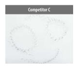
Cutting conditions: Vc = 400 m/min, ap = 0.5 mm, f = 0.15 mm/rev, Wet, CC \*\* 09T304 type Workpiece: AlMg1SiCu
