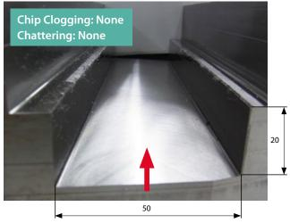
Cutting conditions : Vc = 40 m/min, ap  $\times$  ae = 20  $\times$  50 mm (Slotting), fz = 0.08 mm/t ø50 (5 Flutes), wet (external and internal coolant), workpiece: Ti6Al4V Machine: BT50
