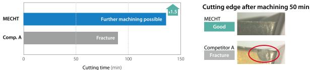
Cutting conditions: Vc = 40 m/min, ap × ae = 43 × 20 mm, fz = 0.12 mm/t , ø50 (5 Flutes), wet (external and internal coolant), workpiece: Ti6Al4V Machine: BT50
